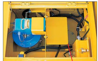
Grease can drum storage location
