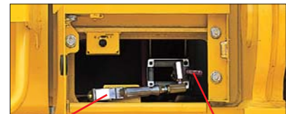
Grease gun The grease gun can be reached from ground level. Indicator
